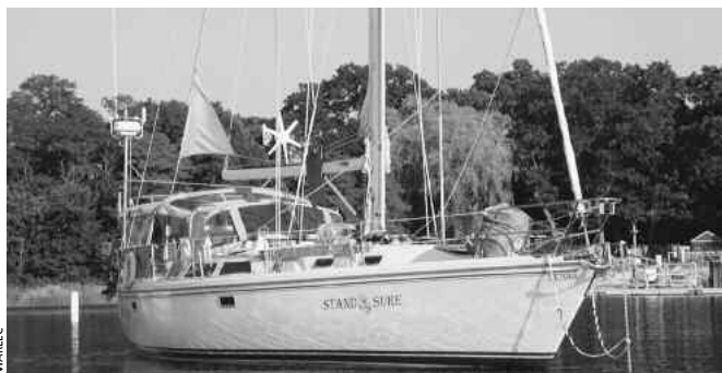
Fig. 5.5: Microturbines. Many microturbines like the Marlec (shown here) have no governing mechanism to slow the rotor in high winds. They rely on the relatively low rotor speed and rugged construction to endure high winds.
