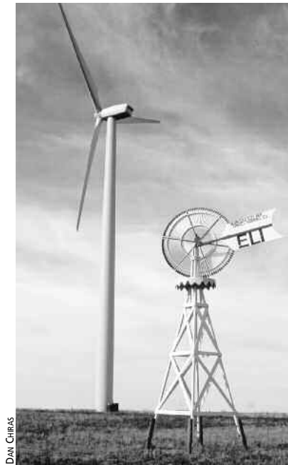
Fig. 1.1: The Old and the New. Water-pumping windmills like the one in the foreground were once common in the West and Midwest. The technology hasn't changed in 100 years. In the distance is a modern commercial wind turbine that generates electricity to power cities and towns.
