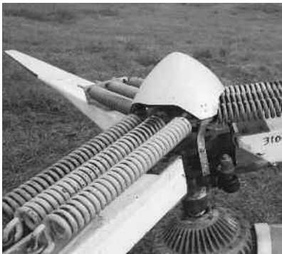
Fig. 5.9: Pitch Control — Blade-Actuated Governor. Numerous ingenious methods of blade pitch control have been devised. In this turbine, a Jacobs 31-20, the springs are part of a complex and effective blade pitch control mechanism.
